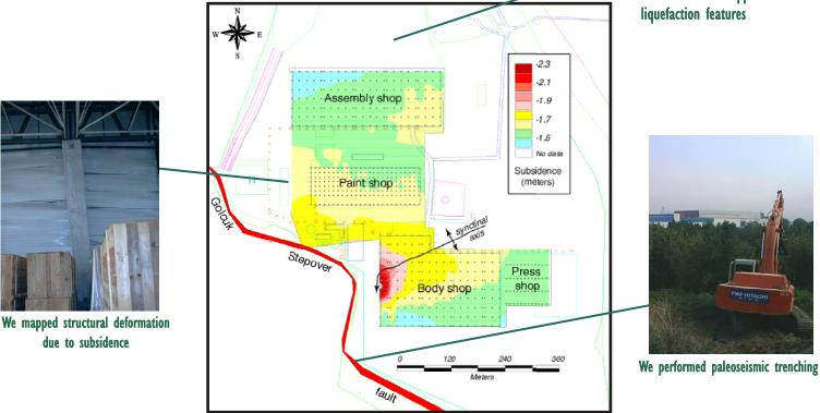
Geologic field mapping of the fault zone and quantitative analysis of subsidence in the area of the buildings
