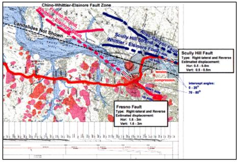
Sample map from our report showing the pipeline alignment, landslides, active and potentially active faults, and potential liquefaction zones. All the mapping was prepared in a GIS environment with comprehensive data tables for each mapped feature. Poster prints were made for State-agency presentations.
