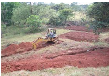
3-D trenching of a feeder channel across the Gatún fault to measure slip per event and timing of past events.
