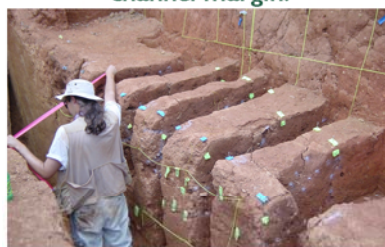
2-D and 3-D trenching of the Gatún fault to measure fault displacement of a 2500-3000 ka channel margin.
