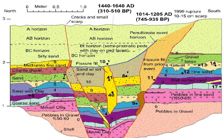
Excavations across small, surface fractures revealed a pattern of prior, larger paleoseismic offsets.
