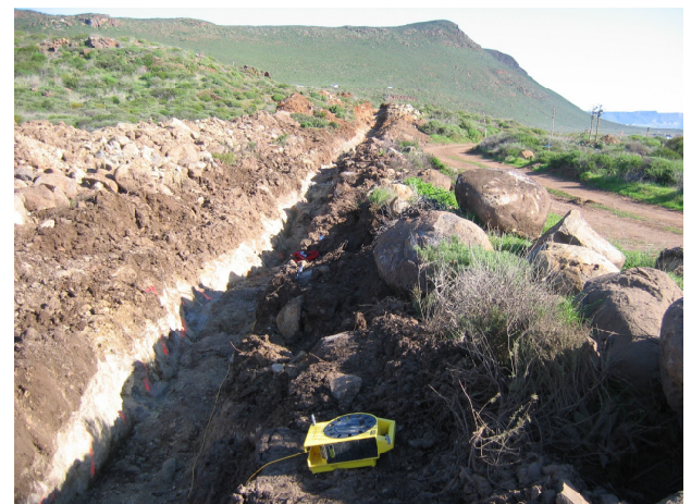
Figure 3. Fault trench exposing marine terrace (boulders) overlying basalt.
