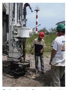
The Cone Penetration Tests were advanced into the ground using a track-mounted drill rig modified to accommodate the CPT rods. Digital measurements were recorded by and saved to a field laptop computer. Processing of the CPT data was done in the evenings allowing us to modify our field program as necessary in response to the day's findings.
