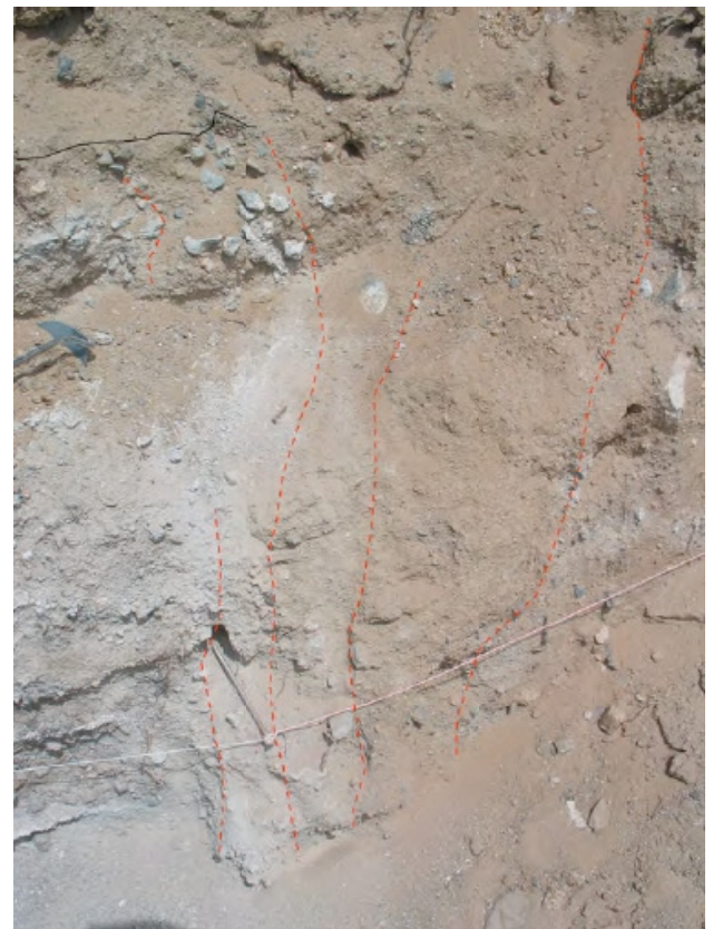
Top: Photo of the entire fault zone exposed, showing the truncation of the Stage IV carbonate horizon. Based on the carbonate stage development, we estimated these deposits at ~100,000 years old.
