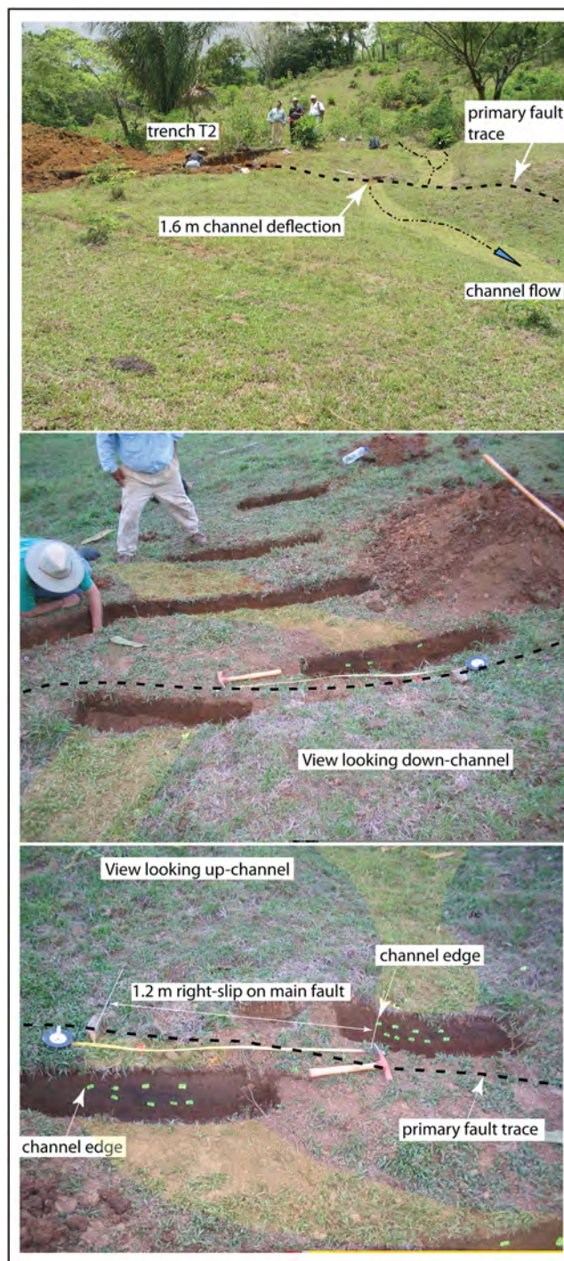
Figure 6. Interpreted photographs of the small, 1.6–2 m offset swale, located a few meters north of trench T2. Several small trenchettes (Fig. 3d) exposed a charcoal-bearing buried channel from which we resolved a minimum of 1.2 m of brittle slip on one of the fault strands. The swale is deflected 1.6 m, with a maximum of about 2 m. The color version of this figure is available only in the electronic edition.
