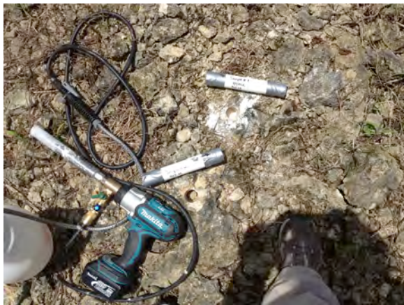
Fig. 8: Sampling drill used for the older coral platforms.
