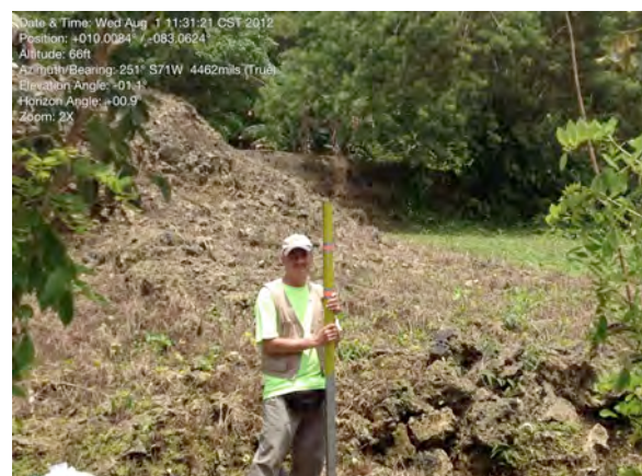
Fig. 6: Example shot of the theodolite surveying of the relative vertical separation between the coral platforms.
